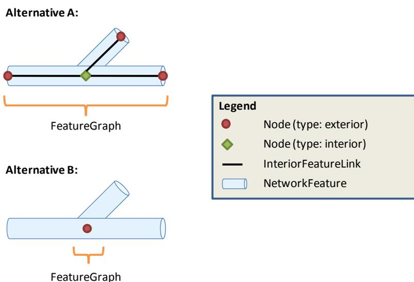
**Fig. 4:** two alternative graph representations for one single *\_NetworkFeature*
