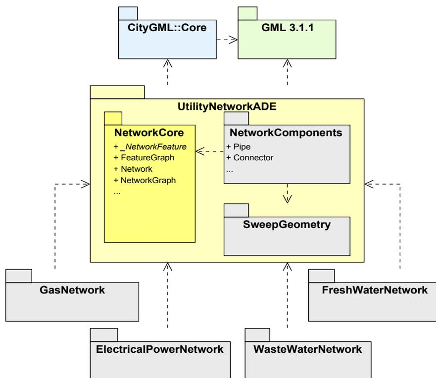
Fig. 1 Package diagram of UtilityNetworkADE
