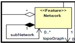
Accordingly a network inherits the attributes for the modeling of a unique ID, as well as a description and a name. Further attributes are not yet intended in the actual draft version of this data model.
